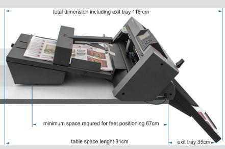
The system comprises three separate components: inserter, cutting plotter and exit tray. These three parts are positioned one above the other and they must be positioned on a table, where the exit tray may be left hanging above the edge. The exit tray extends for 35 cm and must be positioned in a location free of tight
